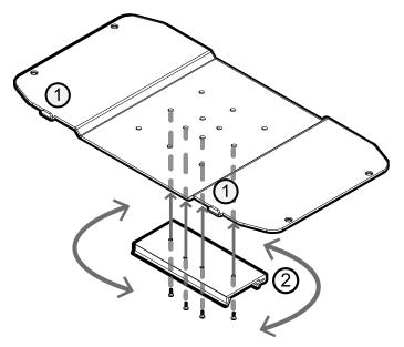
$\textcircled$  Indicates the tabs on the mounting plate which fit in to the slots on the rear of the appliance.
