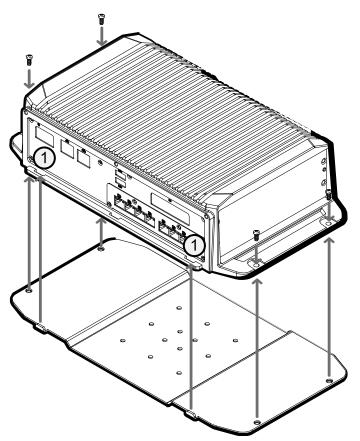
0 Indicates the slots on the rear of the appliance into which the tabs on the mounting plate fit.
