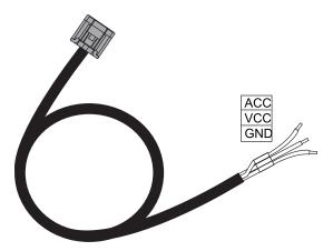
To make a permanent power connection (unswitched), connect both the ACC and VCC wire to the positive side of the power source. Connect the ground wire to the ground side of the power source.
