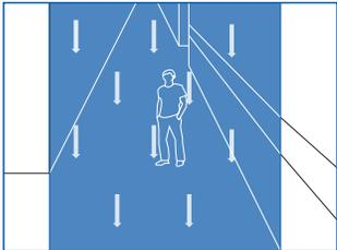
The event is triggered when a person or vehicle moves in the prohibited direction of travel.
