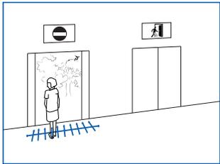
The event is triggered when the specified number of persons or vehicles cross the directional beam that is configured over the camera's field of view. The beam can be unidirectional or bidirectional.
