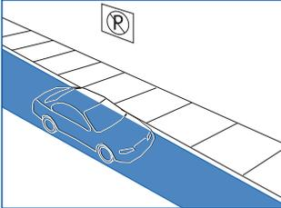
The event is triggered when a person or vehicle in a ROI stops moving for the specified threshold time.
