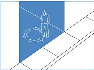
The event is triggered when a person or vehicle stays within a specified ROI for the specified duration.
