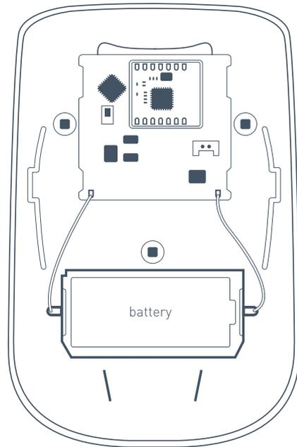
PICTURE 5. Sensor with the top cover removed
