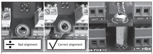
The connector on the IPCard <u>MUST align properly</u> with the connector on the main board, and mounting holes in the IPCard must align with spacers before attempting to install the screws.
