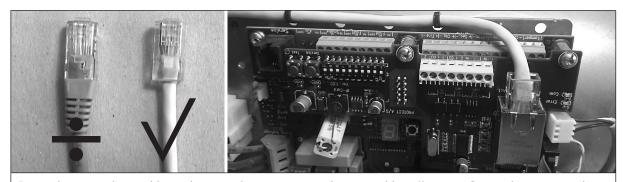
Route the networking cable as shown in the picture to make sure cable will not conflict with any internal part of the fog cannon. Let the network cable exit the hole in the cabinet used for any other normal signal cable to and from the alarm system.
