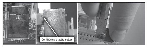
On some fog cannon units a service connector on the main PCB may have to be modified to give space enough to install the IPCard.
