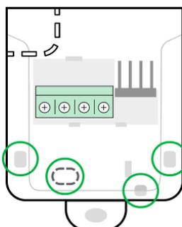
4. Run the cable from the hub into the detector's body through the hole made.
