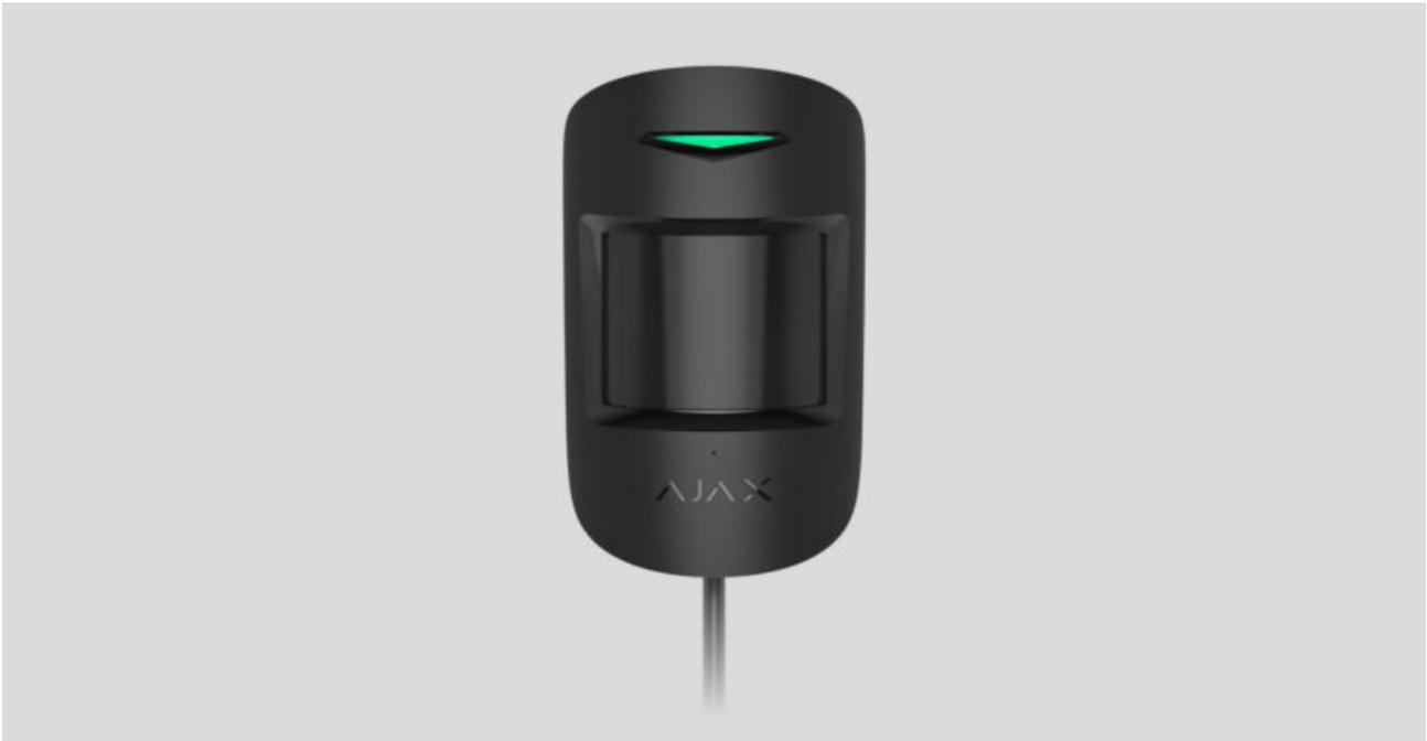
**CombiProtect Fibra** is a wired motion and glass break detector. Detects movement at a distance of up to 12 meters and glass break at a distance of up to 9 meters. Together with the IR sensor, it applies a radio-frequency scan that filters out thermal interference.
