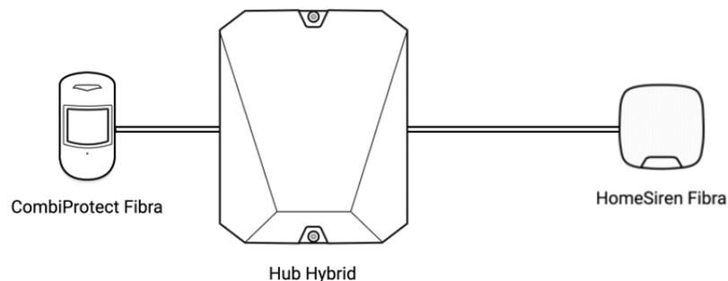
CombiProtect Fibra is a wired motion and glass break detector. In the armed mode, the detector instantly transmits an alarm signal to the hub when it detects movement or break. The hub, in turn, activates the sirens connected to the system, launches scenarios, and notifies users and the security company.
