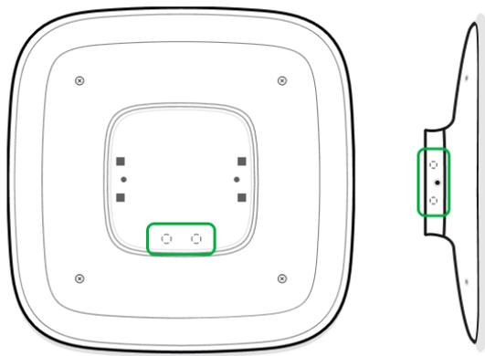
4. Run the cable from the hub into the siren body through the hole made.
