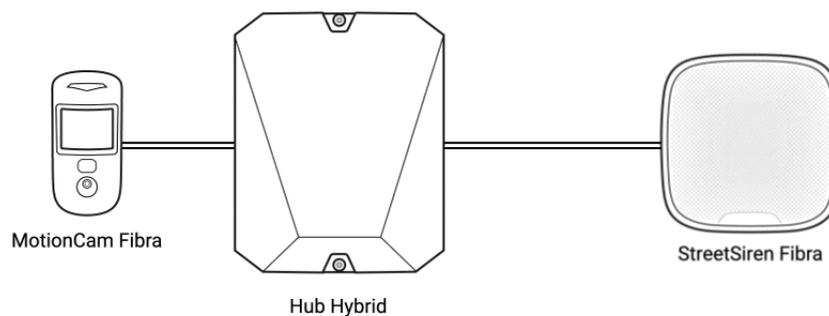
StreetSiren Fibra is a wired outdoor siren. The device is equipped with a piezoelectric buzzer for sound alerting and an LED frame for visual alerting.
