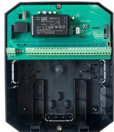
MultiTransmitter comes in a protective container with a dedicated space for a rechargeable battery.
