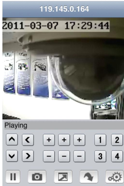
**Button definition:** 【PTZ direction control (left, right, up, down)】; 【area select (zoom in, zoom out)】; 【focus (+, -)】; 【aperture (+, -)】; 【snapshot】.
