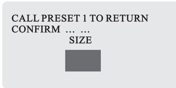
Using up, down, left and right key to adjust the size of the mask, then call preset 1 to confirm and return.
