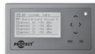
As a rule of thumb, the signal level goes down by 6dBm for every time range is doubled in a free air line of sight environment.
